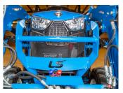
Standard Factory Grille Guard W/ Loader Full Length Grille Guard Protect Body Panels And Radiator
