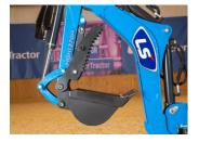
*Optional Thumb Configuration Backhoe* Provides Added Functionality To The Heavy-Duty Backhoe
