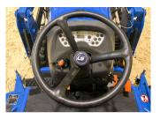
*Standard Tilt Steering* Provides Enhanced Operator Comfort
