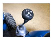
**Integrated Joystick Provides Comfortable Access** For Loader Operations. 3rd Function (Option)
