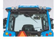
Four Standard Rear Worklights Provides Significant **Illumination During** Night Operation
