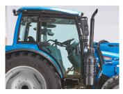
Right-Side Cab Access **Enables Operators To Access** Both Sides Of The Cab (Door And Steps)
