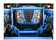
Standard Factory Grille Guard W/ Loader Full Length Grille Guard **Protects Body Panels** And Radiator
