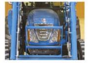
Standard Grille Guard With Loader And Position ROD Protects Grille And Radiator In Loader Applications
