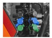
Available With Three Rear Remotes (Cab Only) Provides Added Flexibility For Attachments And Implements
