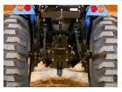
High Capacity Three Point Hitch Heavy-Duty Frame And Lift Cylinders Enable Three-Point Lift Capacity Up To 2,910 lbs.
