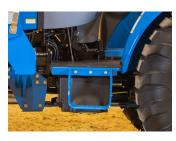
Accessibility Easy Access Platform Via Standard Step And Rubber Matted Surface
